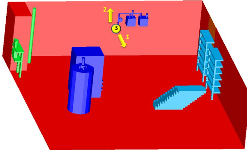
**Figure 8. Basement layout and natural gas leak scenarios.**
