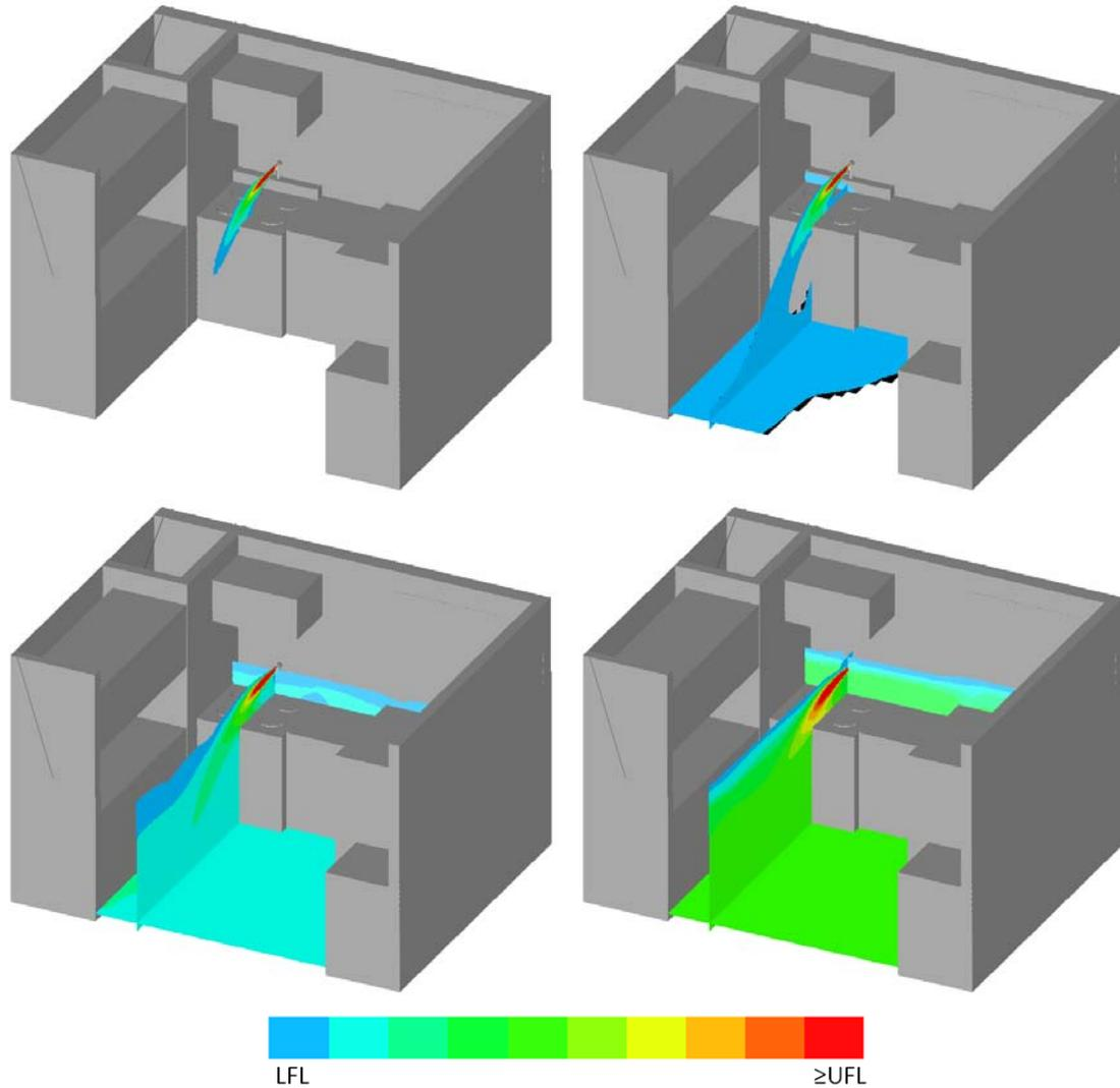
**Figure 4. Propane cloud concentration from free jet leak, after: 5 minutes (top-left); 15 minutes (top-right); 30 minutes (bottom-left); and 60 minutes (bottom-right).**
