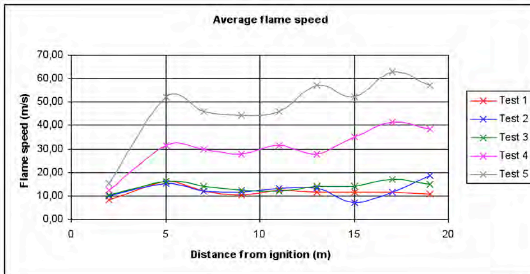
Figure 11: The average flame speed as a function of the distance from the ignition source.
